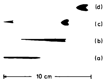
Fig. 2. Thin layer chromatogram of copolymer A (a), copolymer B (b), PMMA- g -oligoamide-A (c), and PMMA- g -oligoamide-B (d) obtained with phenol-chloroform (30:70 by vol).
